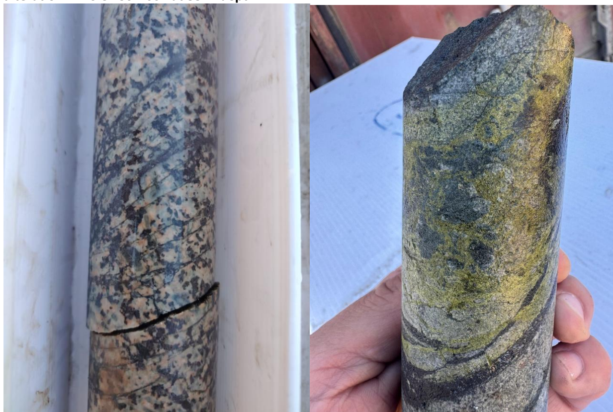
Figure 3. Photos of core showing potassic alteration in hole 25SB-004 at 300 m depth and propylitic alteration in hole 25SB-002 at 88 m depth.
