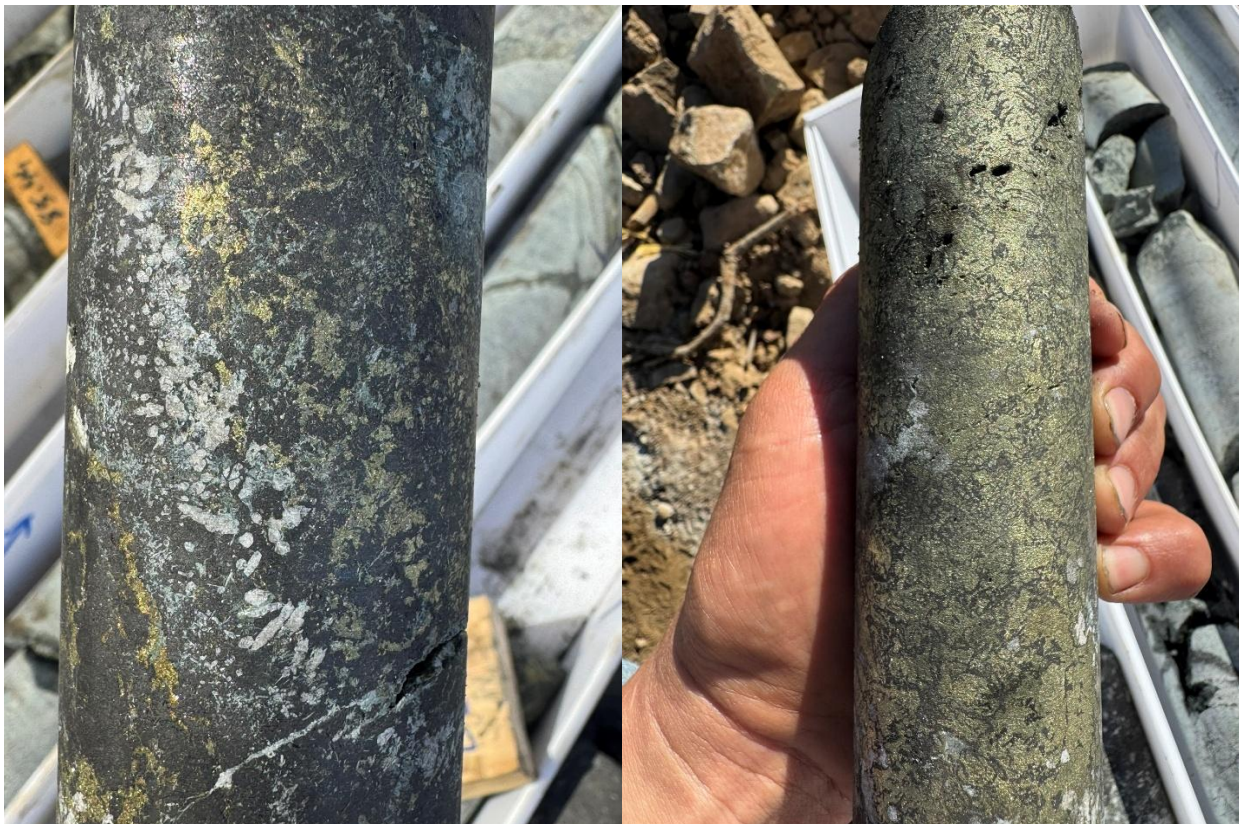
Figure 2. Photos of core from holes 25SB-002 and 25SB-004 showing the relative concentration of magnetite vs chalcopyrite and gangue minerals (apatite and chloritized actinolite) in the vein.
